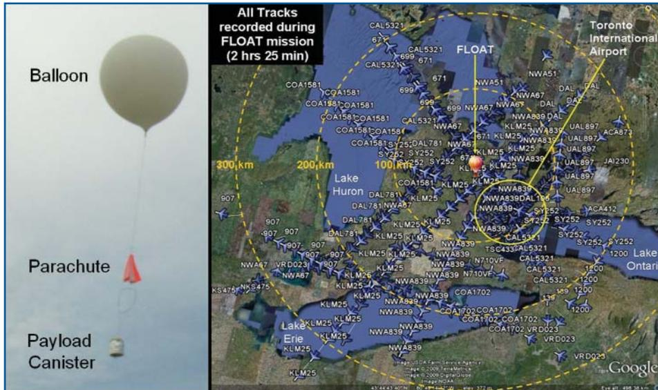
Fig. 1 FLOAT is shown a few minutes after launch. During the 2.4 hour flight all ADS-B equipped aircraft within a 200 km radius of the balloon were detected. A total of 2,076 unique messages were received by the payload.
