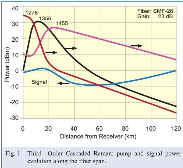
Fig. 1 Third Order Cascaded Raman: pump and signal power evolution along the fiber span.
