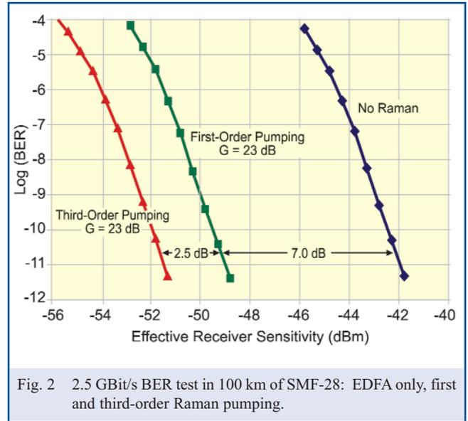
Fig. 2 2.5 GBit/s BER test in 100 km of SMF-28: EDFA only, first and third-order Raman pumping.
